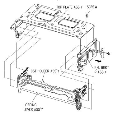
Fig.3-2 DISASSEMBLY OF THE FRONT LOADING ASS'Y
